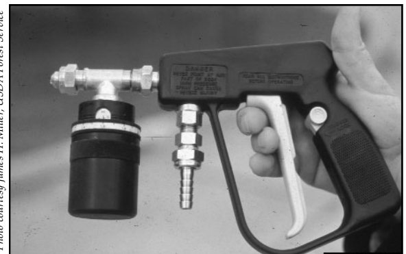
Meter-Jet handgun for spot application of herbicides
